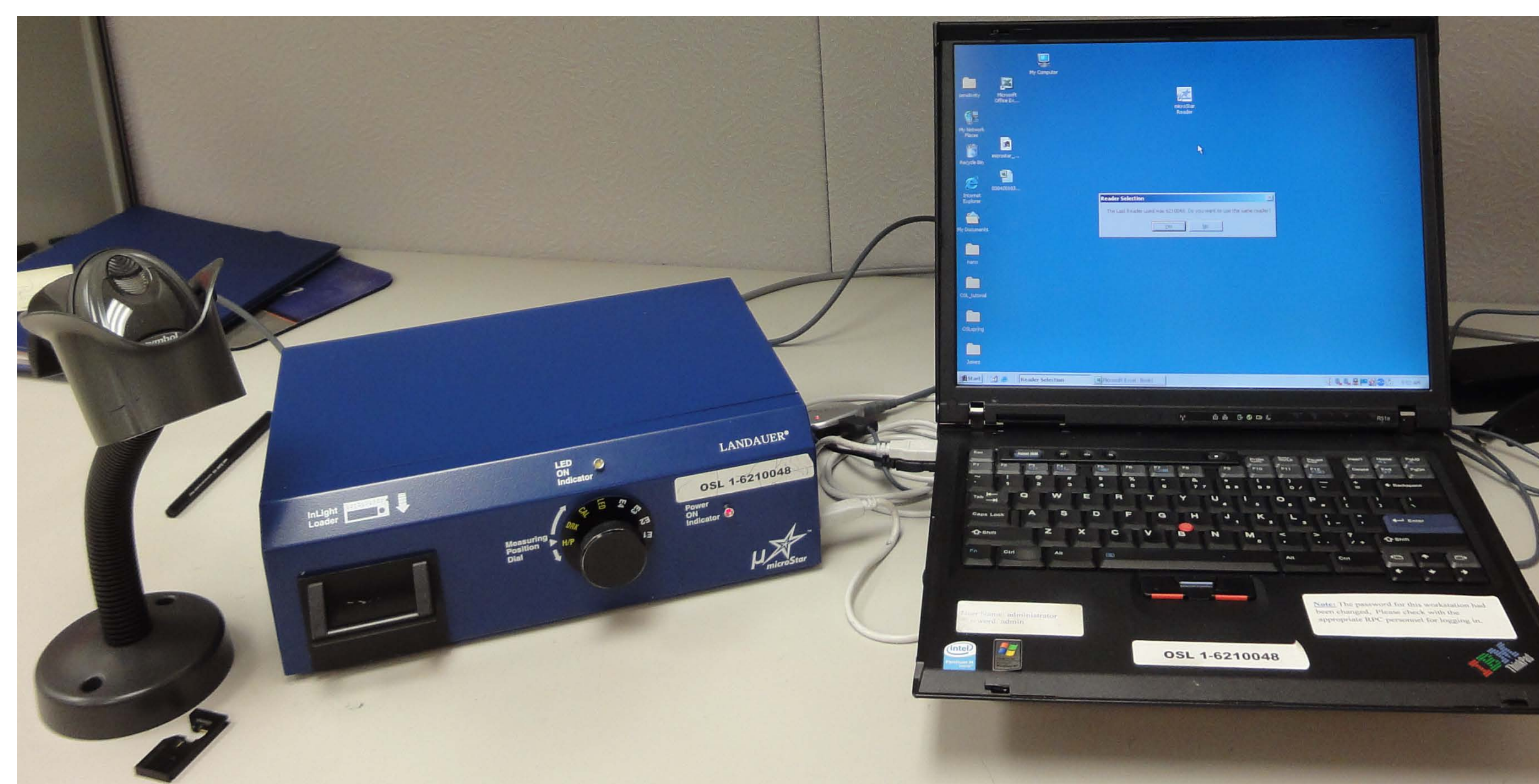
Figure 1: MicroStar ® reader. Computer, scanner and adapter for nanoDot TM are shown in picture
