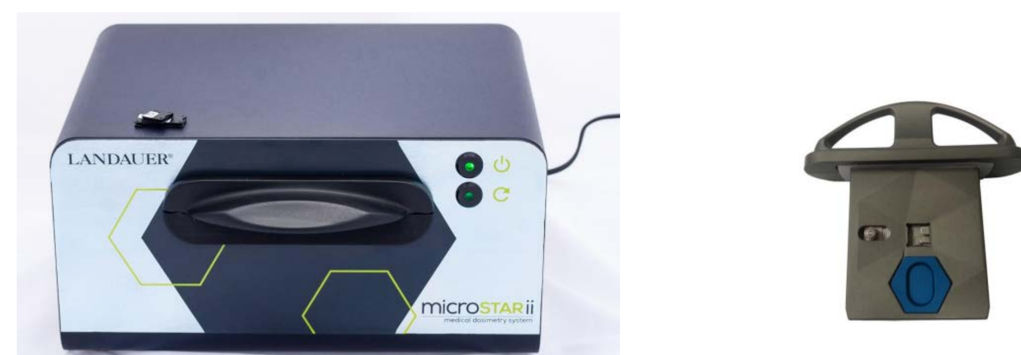
Figure 2: microSTARii TM reader and drawer for nanoDot TM readings
